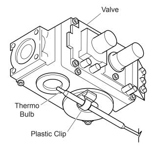
Figure 13 - Clipping Thermo Bulb into Plastic Clip.
